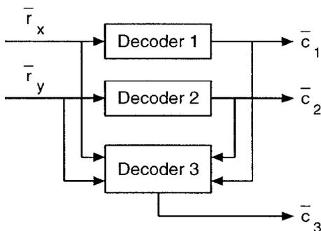
Figure 3: Decoder of three-level coded 8-PSK modulation
