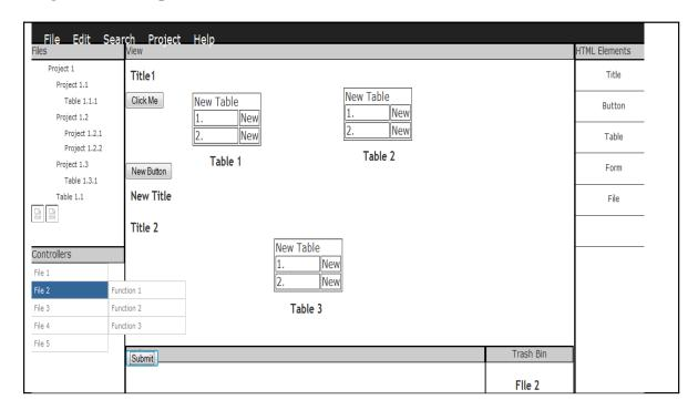
The above figure 3 shows the complete View part of the IDE. As explained above, it has got different divisions performing various tasks. The bottom part of the web page is to delete any files .It can be done by dropping the files onto trash bin.
