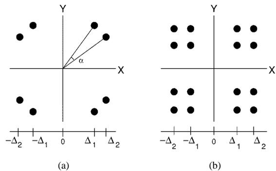
Fig. 1. Nonuniform constellations: (a) 8-PSK and (b) 16-QAM.
