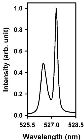
**Figure 3.**  $^5D_1 \leftarrow ^7F_0$  transition excitation spectrum of  $[\text{Eu}((R,R)\text{-}1)_3]^{3+}$  in  $6.67 \times 10^{-3}$  M MeCN at 295 K. The luminescence was monitored at about 615 nm.
