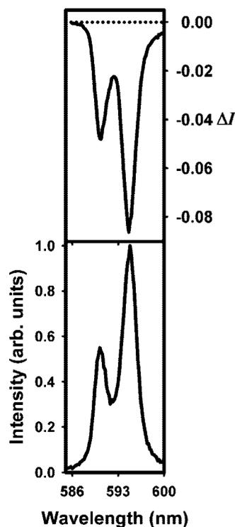
**Figure 2.** Circularly polarized luminescence (upper curves) and total luminescence (lower curves) spectra for the  ${}^5D_0 \rightarrow {}^7F_1$  transition of  $[\text{Eu}((R,R)\text{-}1)_3]^{3+}$  in  $6.67 \times 10^{-3}$  M MeCN at 295 K, following excitation in the spectral range of the  ${}^5D_1 \leftarrow {}^7F_0$  transition.
