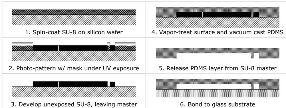
**Figure 1. Process Sequence for Micro Pneumatic Valve**
