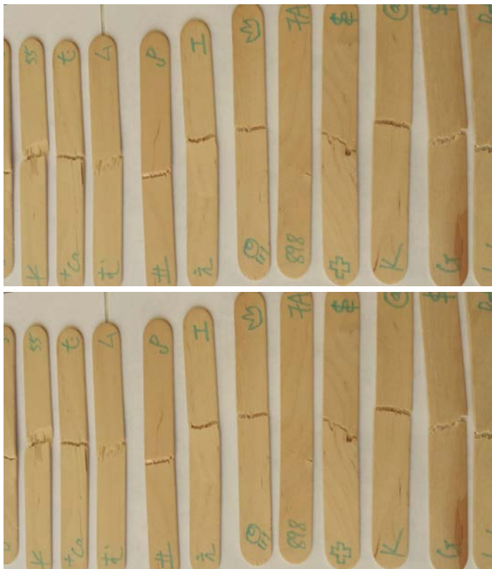
Figure 1. Popsicle sticks with unique fracture patterns reconstituted using physical matching
