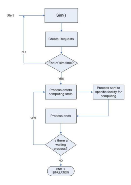
Figure 6.1: simulation model
