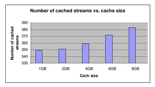
Figure 7.5: number of cached streams vs. cache size
