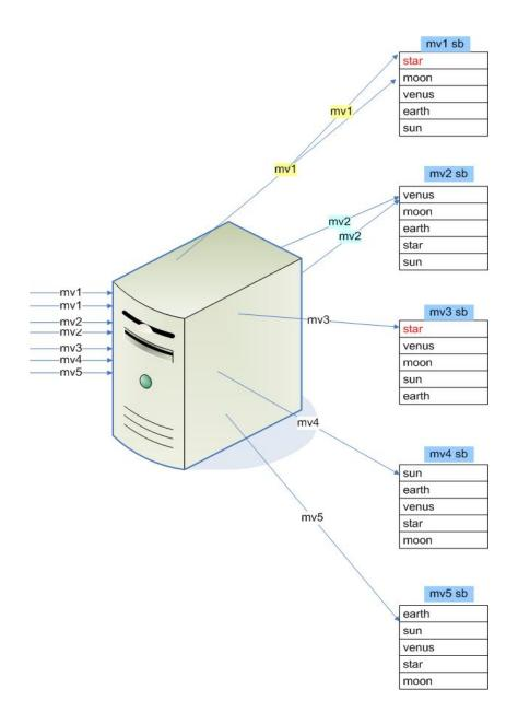
Figure 5.1: request distribution using scoreboard
