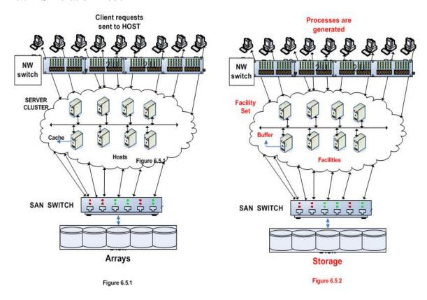
The above two figures explain how we use CSIM in this project. The left figure illustrates our system model. The right figure illustrates the simulation model, in which:
