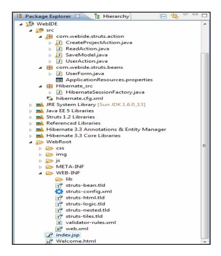
Figure 9. Struts Web Application Directory Structure
