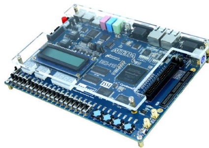
Figure - Altera DE2 115 development board
