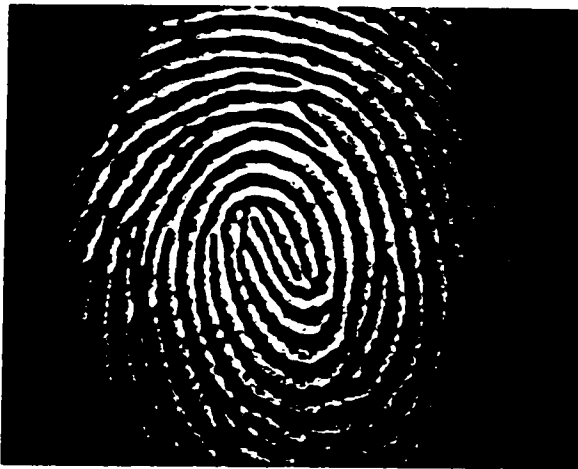
fig 3.4 Fingerprint image through the in line grating sensor
