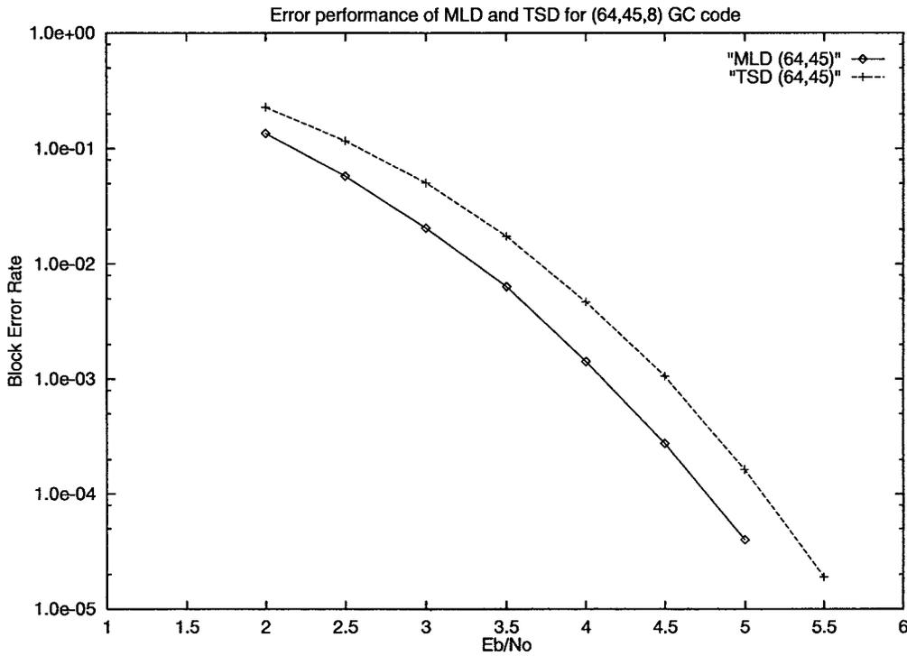
Fig. 3. Simulation results for a binary GC (64, 45, 8) code.
