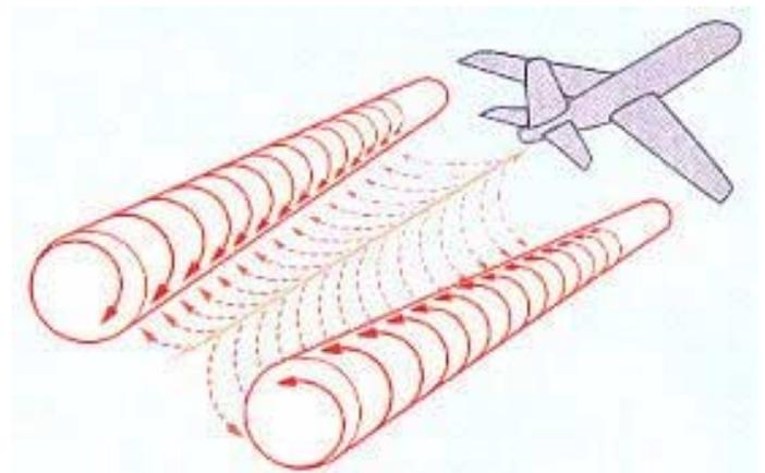
Figure 4: A schematic of the wingtip vortices behind an airplane in flight.
