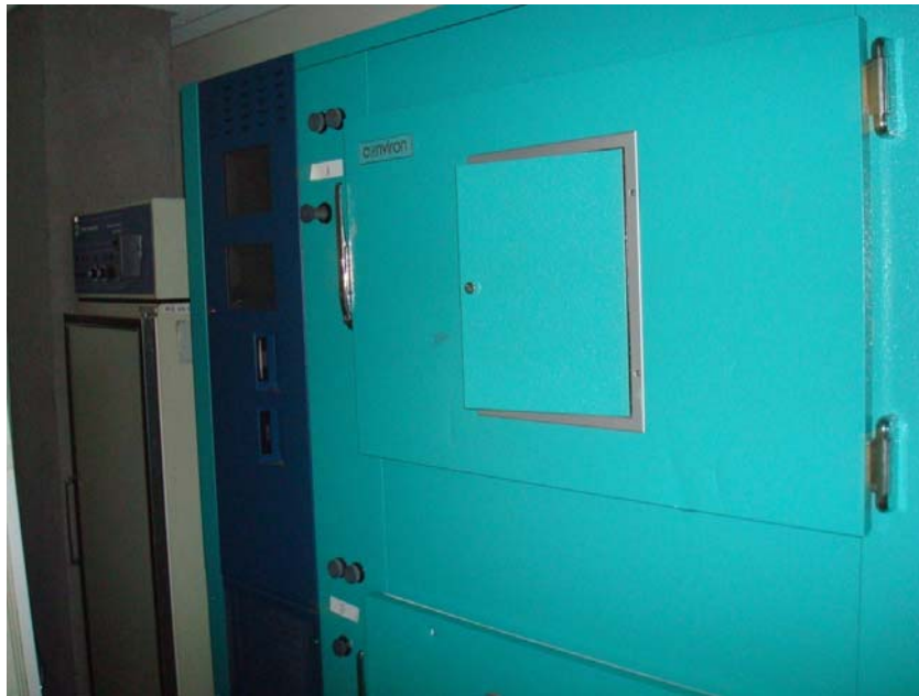
Figure 3 Conviron E7/2 plant environmental chamber
