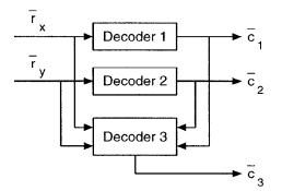
Figure 3: Decoder of three-level coded 8-PSK modulation
