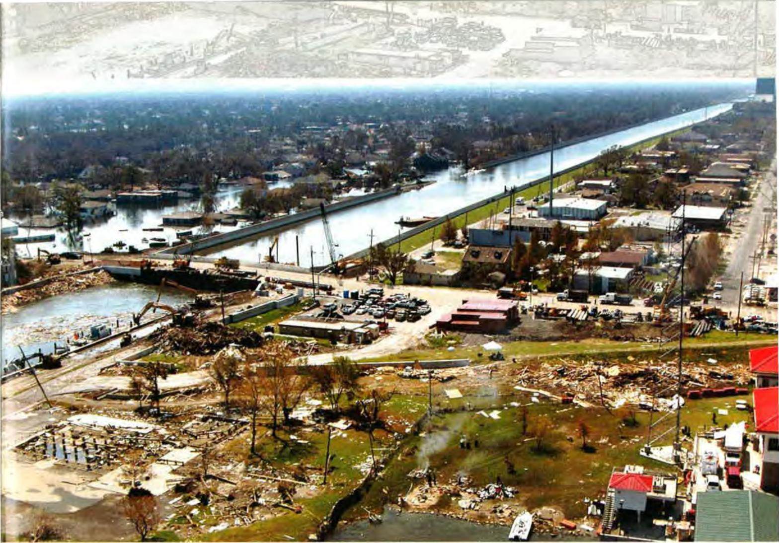
The 17th Street Canal stretches southward between Jefferson and Orleans Parishes in this aerial photo taken Sunday, September 4. The uncompleted bridge in the foreground enabled Corps of Engineers contracts to drive sheet piling to close off the canal from Lake Ponchartrain. Looking down the canal, the breach into Orleans Parish is visible. The skyline of New Orleans lies in the distance. (U.S. Army Corps of Engineers photo by Alan Dooley)
