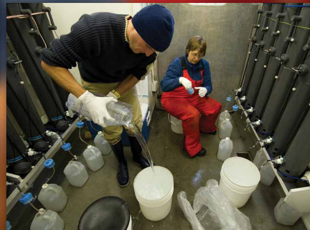
(ABOVE) Rosette with GOFLOs on a Kevlar wire for clean sampling. (LEFT) Shipboard analysis of trace metals in the trace metal container van. (RIGHT) Subsampling GOFLOs in the trace metal container van. Photos © Chris Linder
