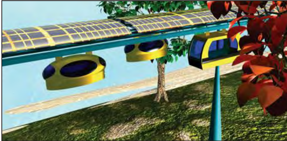
Figure 5. JPods ATN Guideway and Vehicles
