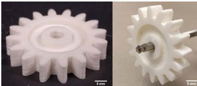
Figure 6. Final spur gear part after sintering.
