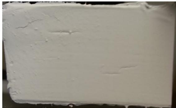
Figure 5. Cracks as a result of fast drying.
