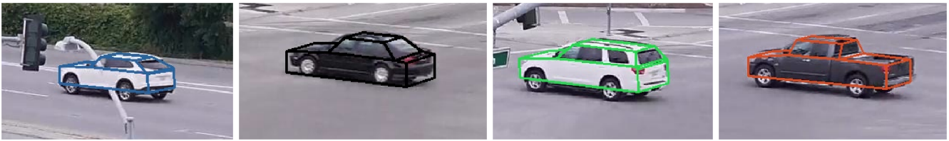
Fig. 9: Team 4 (University of Washington, Seattle): Multiple-kernel based vehicle tracking, segmentation and re-acquisition along with 3D model fitting.
