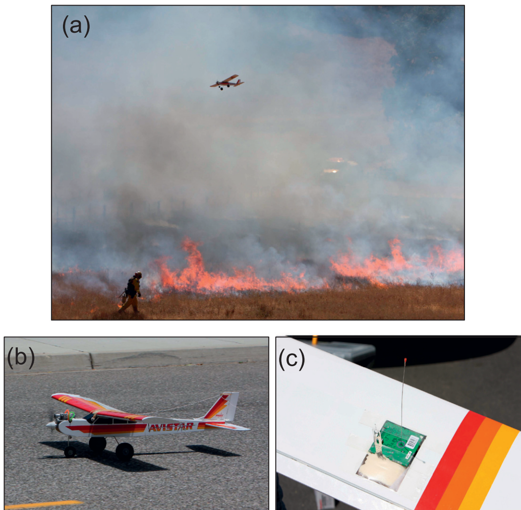
FIG. 1. (a) The miniUAS during the research flight on 7 Oct 2008, (b) completed miniUAS system during the test flight, and (c) Graw, Inc., DFM-06 radiosonde installed in the left wing of the Hobbico Avistar 40. The sensor probe extends below the wing by 10 cm allowing for good exposure to airflow.
