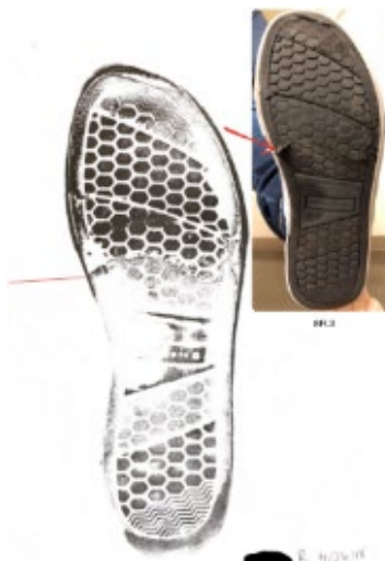
Figure 1. A tear increased in damage between the 2 nd and 3 rd imprints, but it is not easily distinguished in the imprints.
