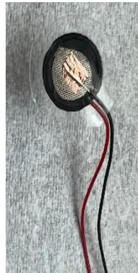
Fig. 12: Piezoelectric pressure sensor.
