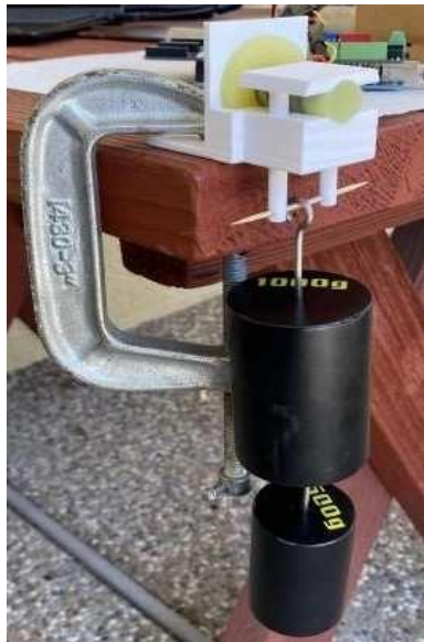
Fig. 15: Apparatus for force sensor calibration.
