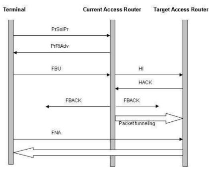
Figure 3. The FMIPv6 handover procedure [8, 11]
