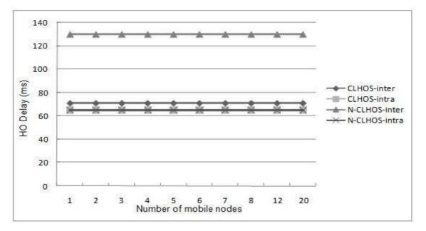
Figure 10. HO Delay via number of mobile nodes
