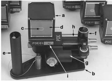
**Figure 1.** USML flight hardware showing pump unit and attached module. For scale; module windows  $\sim 5 \times 5$  cm. a: Plug-in module, b: Pump unit, c: Air-jet orifice, d: Module front window, e: Grip, f: Crank handle, g: Pump piston, h: Compressed-air reservoir, i: Air-valve trigger.
