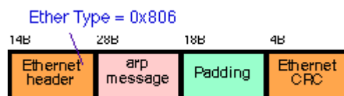
Figure 4: ARP message in an Ethernet header
