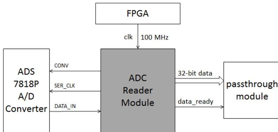
Figure - Block diagram for ADC reader module
