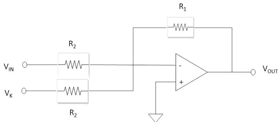
Figure - ECG signal level shifting circuit
