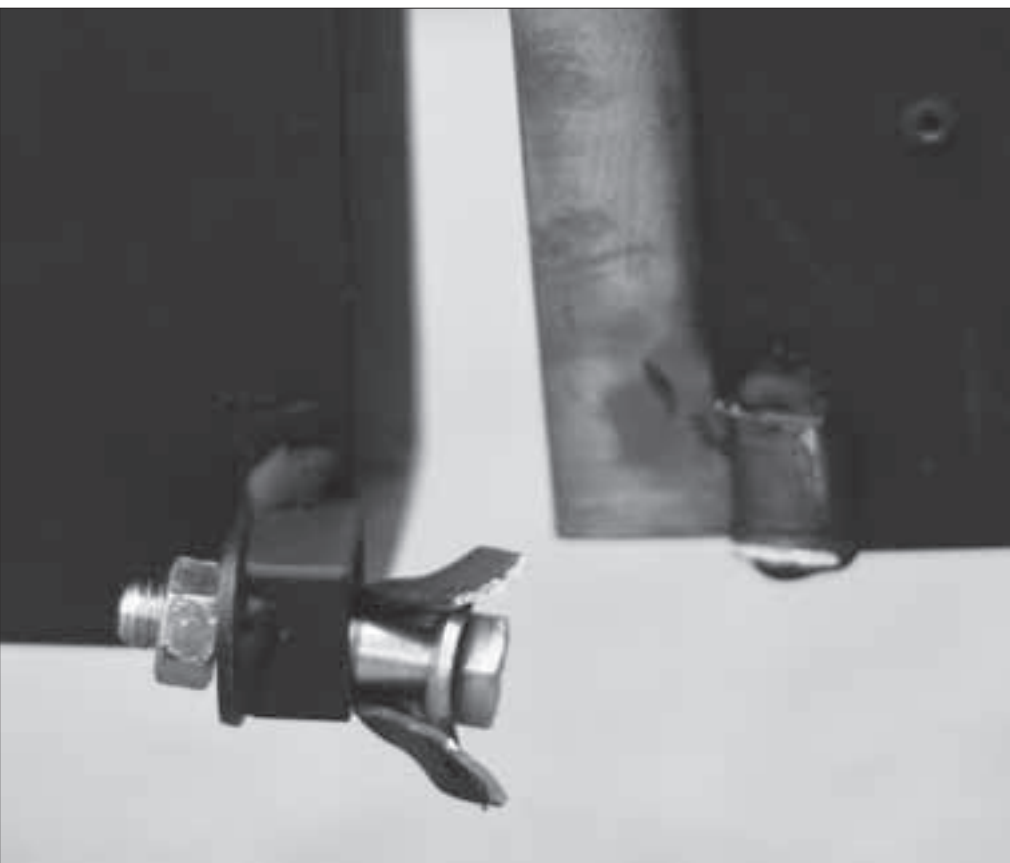
One of the steel connections between two pieces of the bridge ripped, causing a failure of the structure, which collapsed under 1,250 pounds of weight during the vertical load test at the 2010 Mid-Pacific Regional Competition at Chico State University on Saturday (left).
