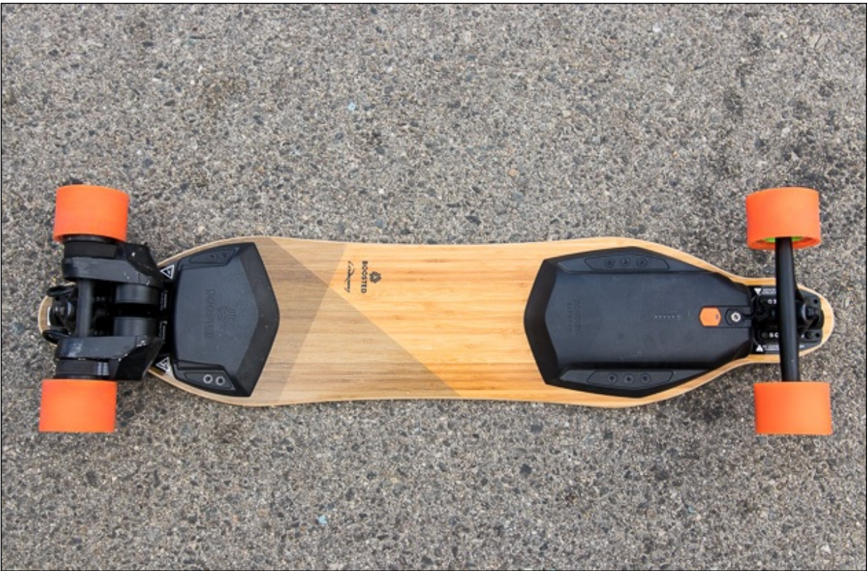
Figure 2. Electric Skateboard (Battery Pack and Drive Components Visible under Deck)
