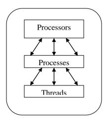
Figure 1. Relationship between processors, processes and threads
