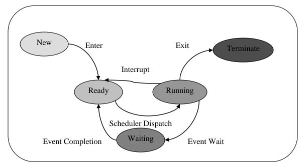
Figure 4. Lifecycle of a thread
