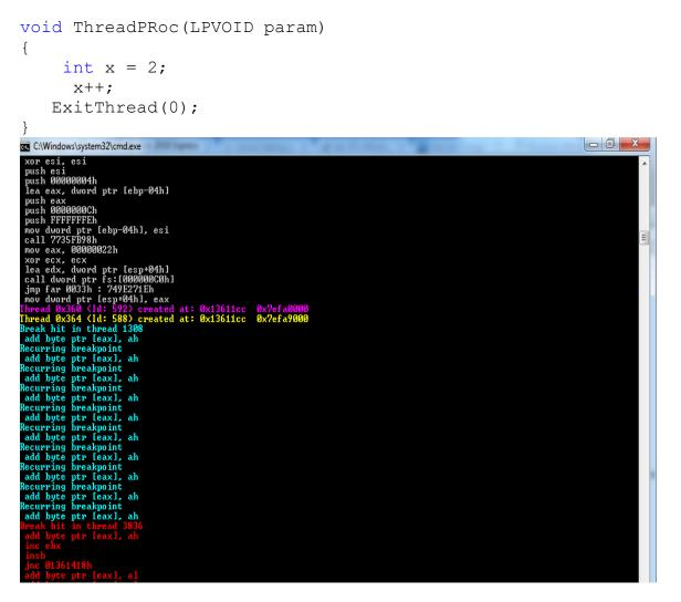
Figure 11. Test case 1 – Simple multithreaded debuggee
