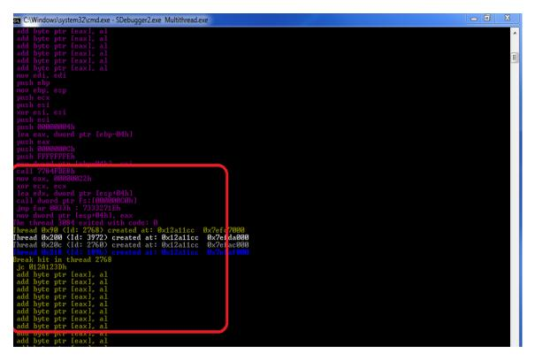
Figure 10. Context switching between threads
