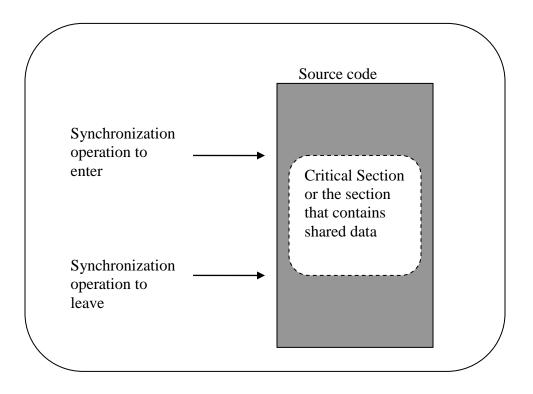
Figure 3. Critical Section and synchronization primitives
