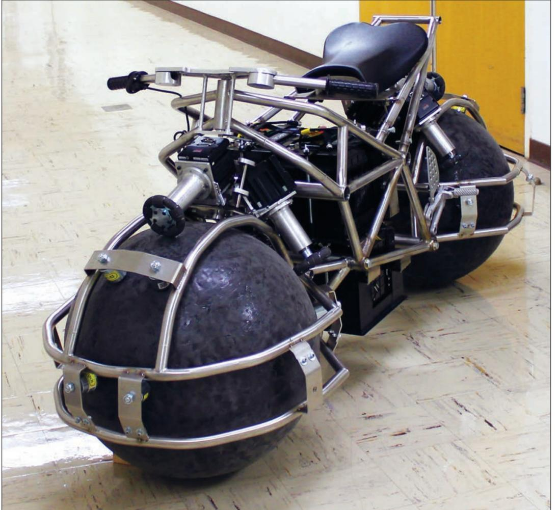
Modeled after the car from the science-fiction film "iRobot," the electric motorcycle is self-balancing and can travel in any direction on a flat surface. **Photo by Jacque Orvis / Spartan Daily**
