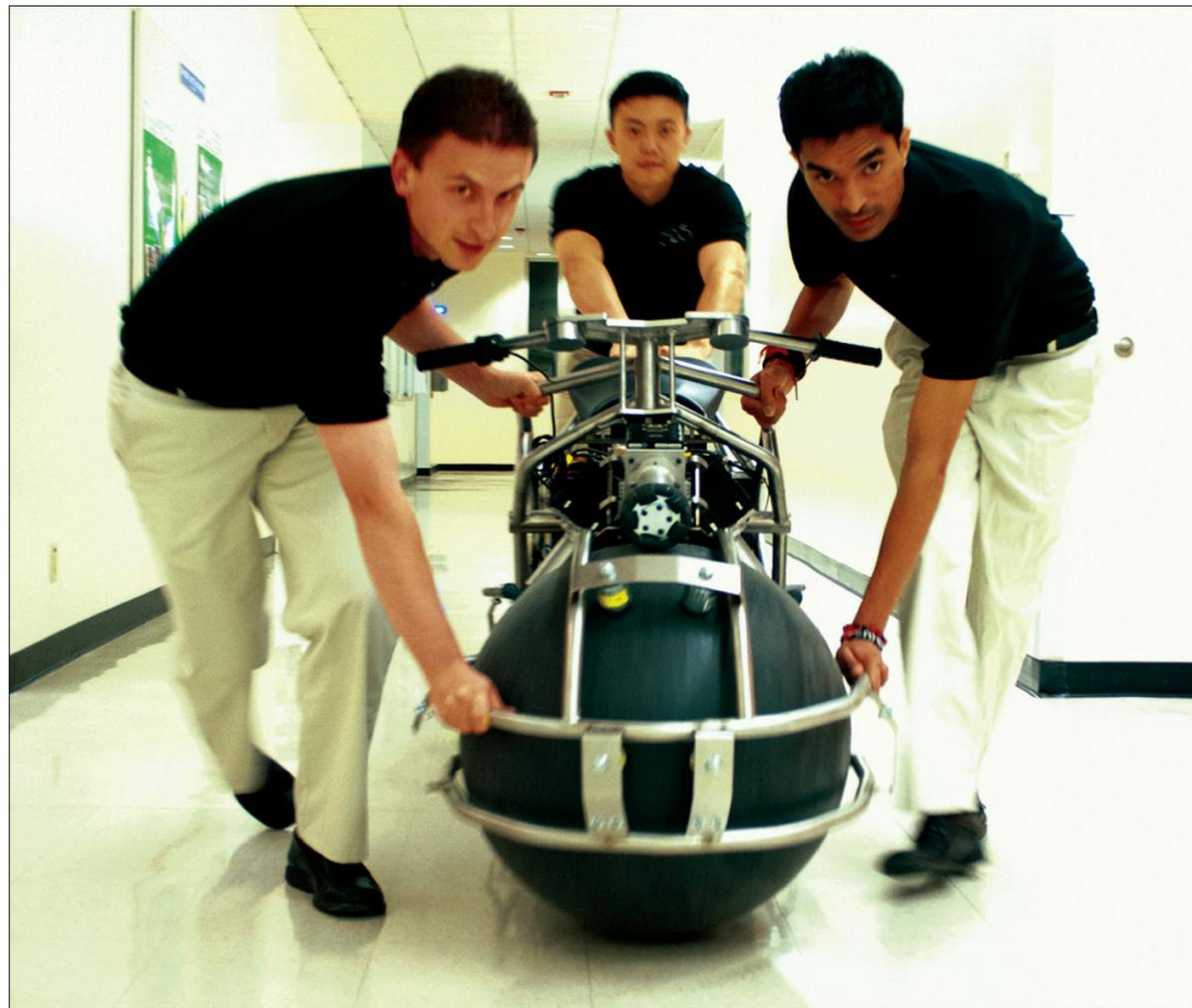
From left to right: SJSU alumni and Spherical Drive System engineers Max Ratner, Henry Li and Andrew Parmar developed a self-balancing, omni-directional, electric motorcycle that rides on spheres. **Photo by Derik Irvin / Spartan Daily**
