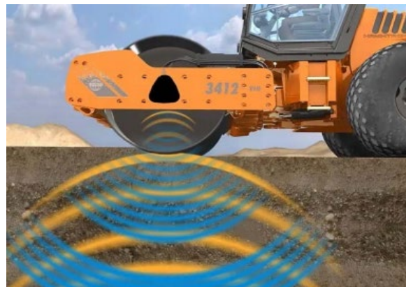
Figure 8. Vibration Response from Soil Layers
