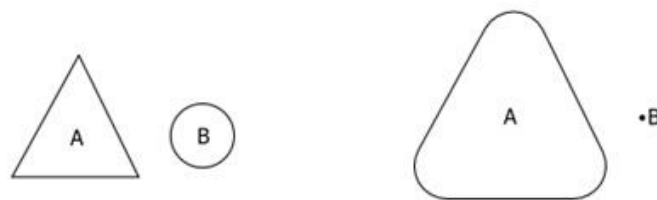
Figure 9. Two polygons on the left and their Minkowski Difference on the right.
