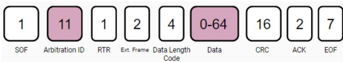
Figure 2. CAN Frame Message Format
