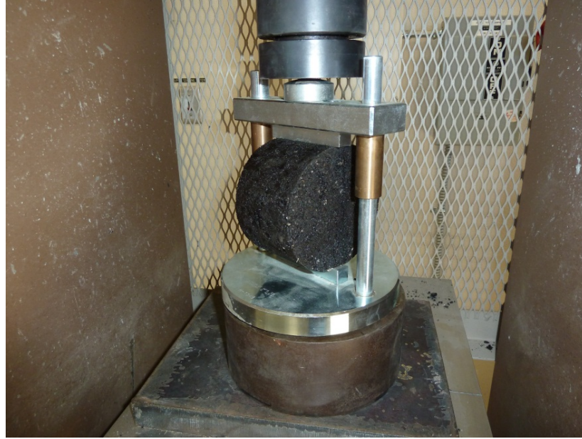
Figure 14. Specimen after Indirect Tensile Test
