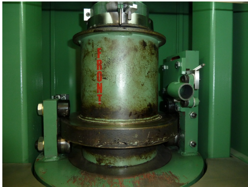
Figure 10. Superpave Gyratory Compactor Ready to Compact a Specimen
