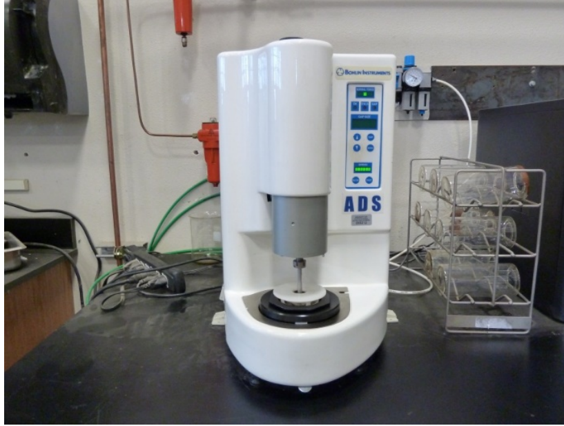
Figure 6. Dynamic Shear Rheometer
