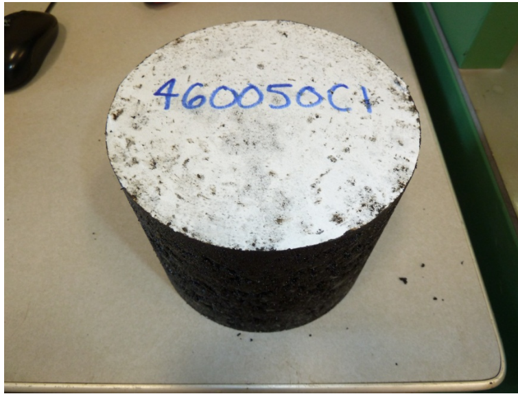
Figure 11. Compacted Trial Specimen
