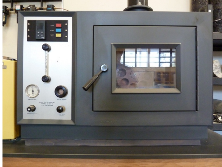
Figure 8. A Rolling Thin-film Oven
