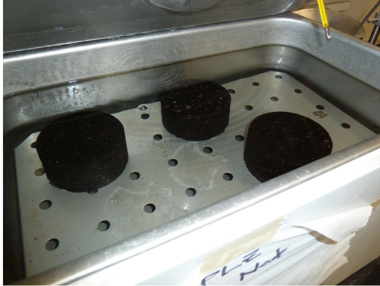
Figure 12. Asphalt specimens Conditioning in Water Bath
