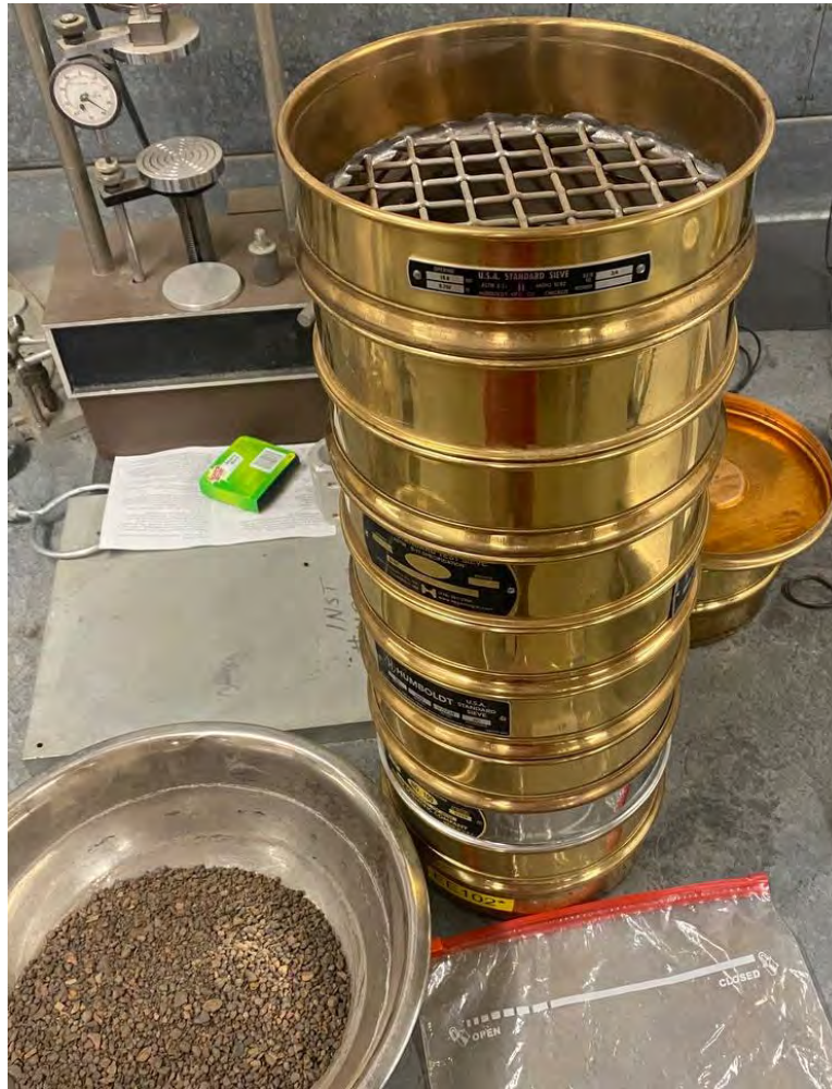
Figure 11. Standard Test for the Sieve Analysis of Coarse Samples (ASTM C136)
