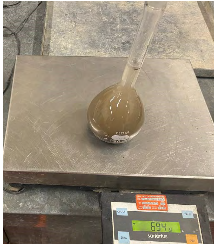
Figure 12. Standard Test for the Specific Gravity of Fine Samples (ASTM C128)
