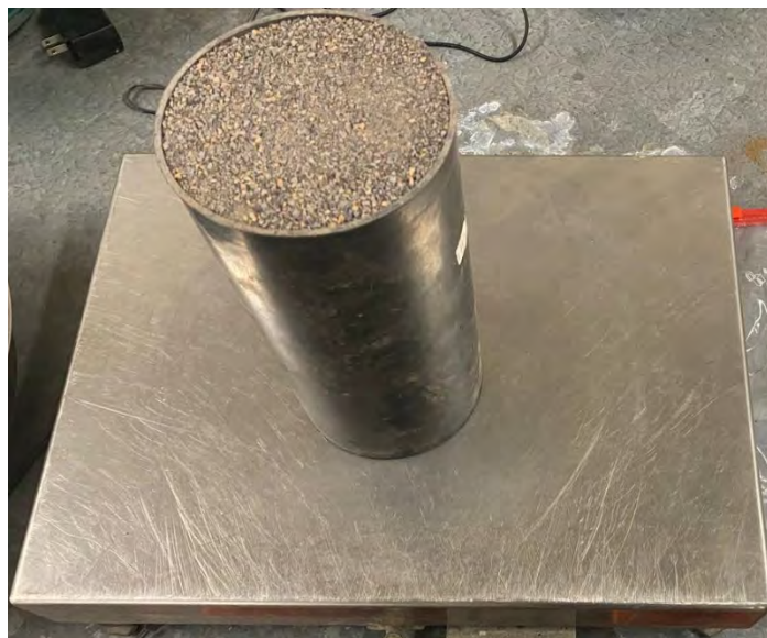
Figure 13. Standard Test for the Bulk Density of Samples (ASTM C127)
