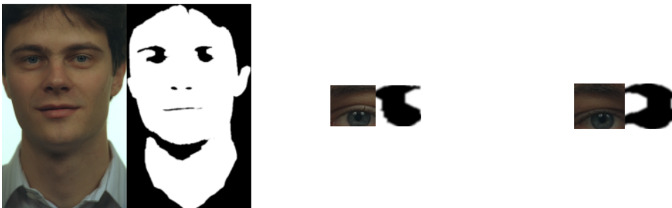
Figure 27: Skin Segmentation Contour Results: The three contours detected by OpenCV showing the face and the two eyes. The left image in each section represents the original image and the right image represents the threshold applied. [26][27]
