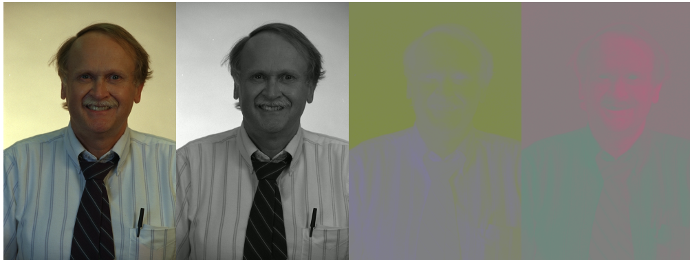
Figure 23: OpenCV RGB Image to YCbCr. The images are from left to right: Original Image, Y-component Image, Cb-component Image, and Cr-component Image. [26][27]
