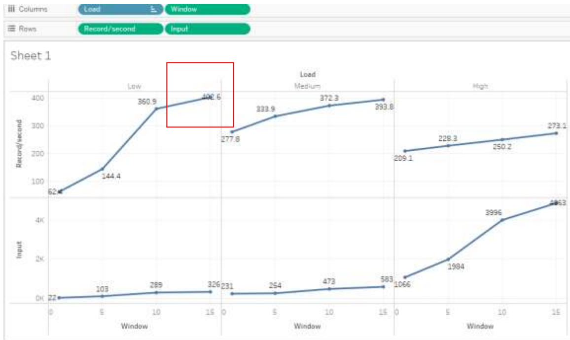
Figure EC2 performance results for spark classifier streaming application
