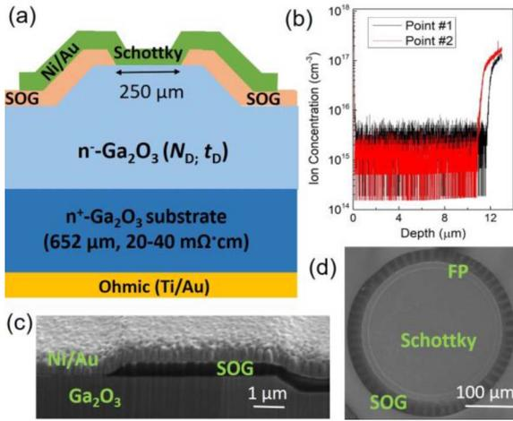
**FIGURE 2.** (a) Schematic of the fabricated vertical  $\text{Ga}_2\text{O}_3$  power Schottky barrier diodes; (b) An exemplary illustration of the drift layer thickness at two spots on the wafer determined by the Si profile measured by secondary ion mass spectrometry. (c) Cross-sectional scanning electron microscopy (SEM) image of the field plate region; (d) Top-view SEM image of the fabricated device.
