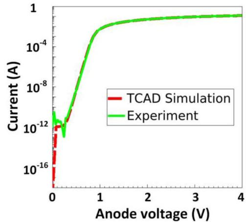
**FIGURE 9.** Experimental  $I$ - $V$  curve and calibrated TCAD  $I$ - $V$  curve showing big difference at  $V < 0.4\text{V}$  due to measurement equipment limitation, despite very good overall calibration.
