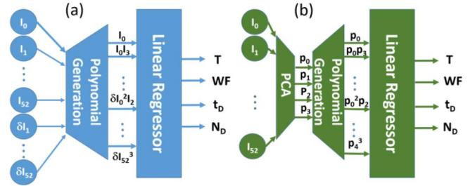
**FIGURE 6.** Schematic of the ML algorithm used in this study. (a) 3<sup>rd</sup> order polynomial generation for “with physical quantities extraction” and (b) PCA followed by 3<sup>rd</sup> order polynomial generation for “without physical quantities extraction”. Meanings of the symbols are explained in Table 3.
