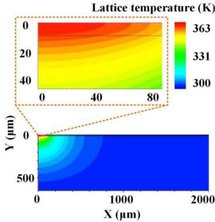
**FIGURE 4.** Simulated temperature distribution at a forward bias of 4 V in the whole simulated structure with cylindrical coordinates (identical to total piece size) and in the zoomed-in anode region.
