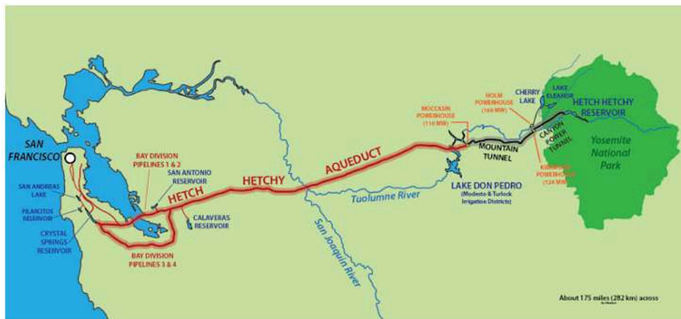
Figure 4: Hetch Hetchy Aqueduct.
