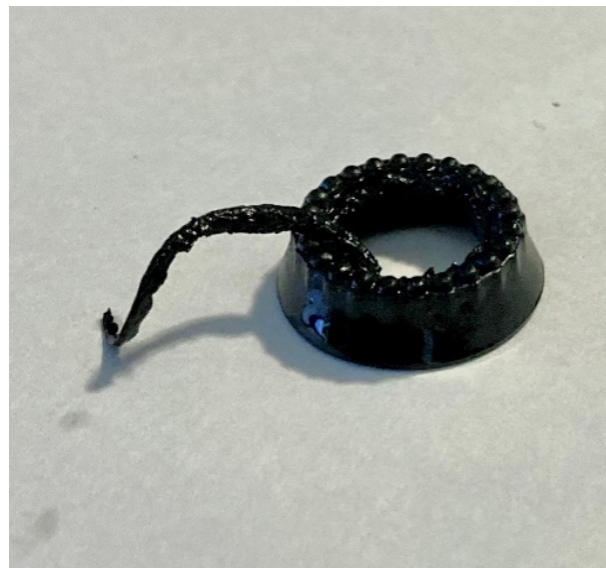
Figure 17. Failure mode of the proportioning valve lower seal during reliability testing.
