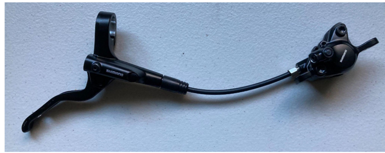
Figure A5. Shortened brake system to eliminate potential hysteresis due to trapped air and hose expansion.
