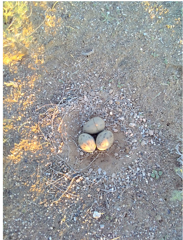
Fig. 1. Egg logger housed inside a 3D-printed and painted artificial egg (uppermost egg) in an Asian houbara Chlamydotis macqueenii nest scrape with 2 real eggs
