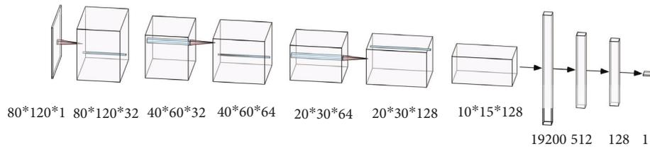
FIGURE 8: M-CNN structure.
