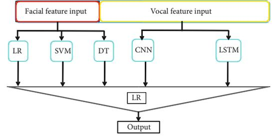
FIGURE 1: FV-Stacking architecture.
