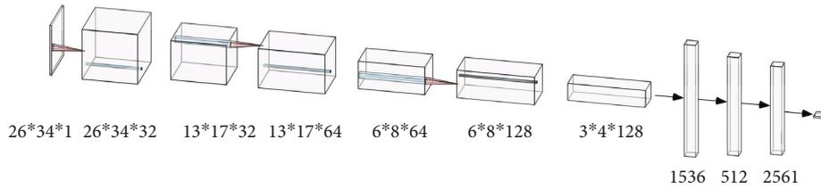
FIGURE 6: E-CNN structure.
