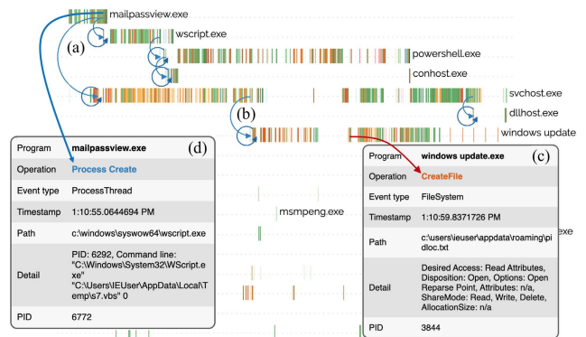
FIGURE 10. MalView view on a Hacktool malware type called Mailpassview . It first creates process svchost.exe (a), then svchost.exe starts windows update.exe (b), and then windows update.exe creates pidloc.txt (c).
