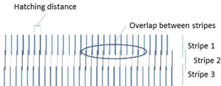
**Figure 1** Illustration of stripe pattern with 5mm stripe width (i.e., length of each vector line) and 0.1mm overlap as scanning strategy used for printing all Ti-5553 and Ti-64 samples.
