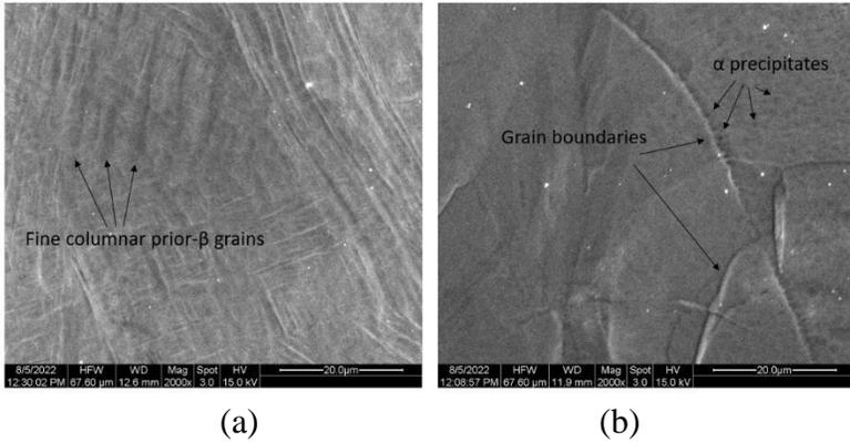
**Figure 4** Higher SEM micrographs of cross sections (i.e., x-y plane, normal to the building direction-z axis) of (a) printed Ti-64 sample showing fine columnar prior- $\beta$  grains filled with  $\alpha'$  martensite inside the cross-section, and (b) printed Ti-5553 sample presenting grain boundaries with  $\alpha$  precipitates appeared in the cross-section.
