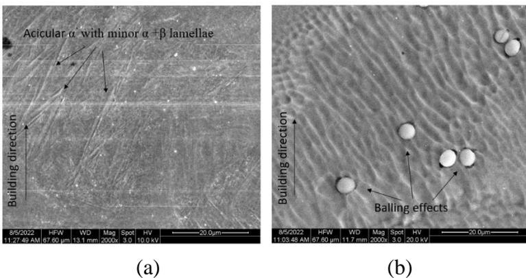
**Figure 5** Higher SEM micrographs of cross sections (i.e., y-z plane, along the building direction-z axis) of (a) printed Ti-64 sample showing acicular  $\alpha'$  phase with minor  $\alpha + \beta$  lamellae randomly organized across the cross-section, and (b) printed Ti-5553 sample presenting the balling effects in the cross-section for the first time.
