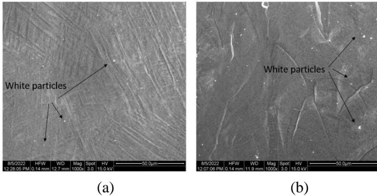
**Figure 3** SEM micrographs of cross sections (i.e., y-z plane, along the building direction-z axis) of (a) Ti-64 and (b) Ti-5553 samples, printed at the laser power of 100 W, a scan speed of 1400 mm/s, a layer thickness of 30  $\mu\text{m}$  and a hatch spacing of 40  $\mu\text{m}$ , respectively, showing more white particles in Ti-5553 compared to Ti-64, indicating higher porosity level in printed Ti-5553 samples than that of Ti-64.
