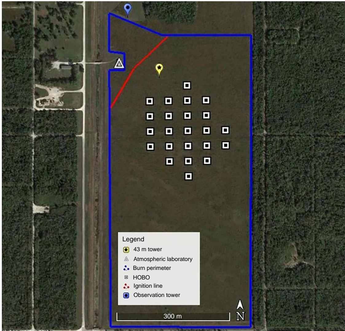
Fig. 9. Map of the experimental design with instrument placement and ignition sequence for the FFII prescribed burn (Google Earth).
