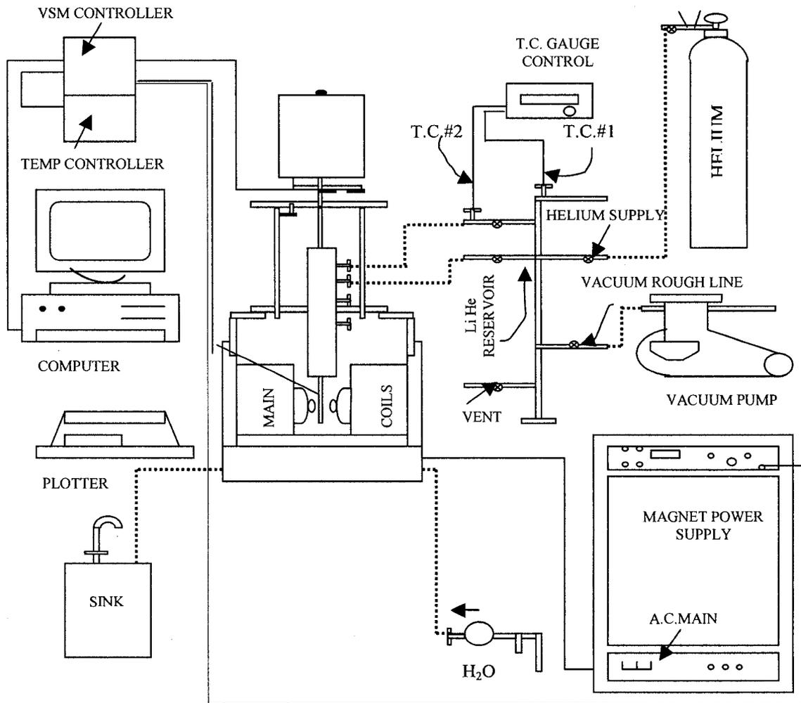
Figure 11. Low temperature VSM schematic
