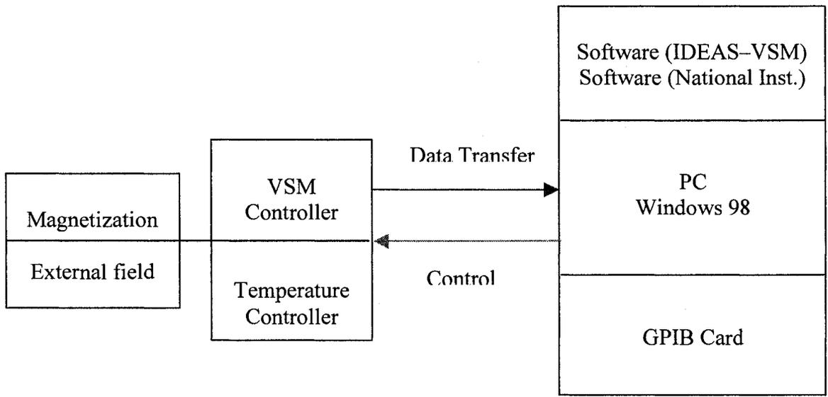
Figure 10. Block diagram of data acquisition.
