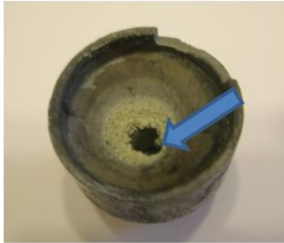
Fig. III-4 Cast nozzle with excessive and non-symmetric erosion
