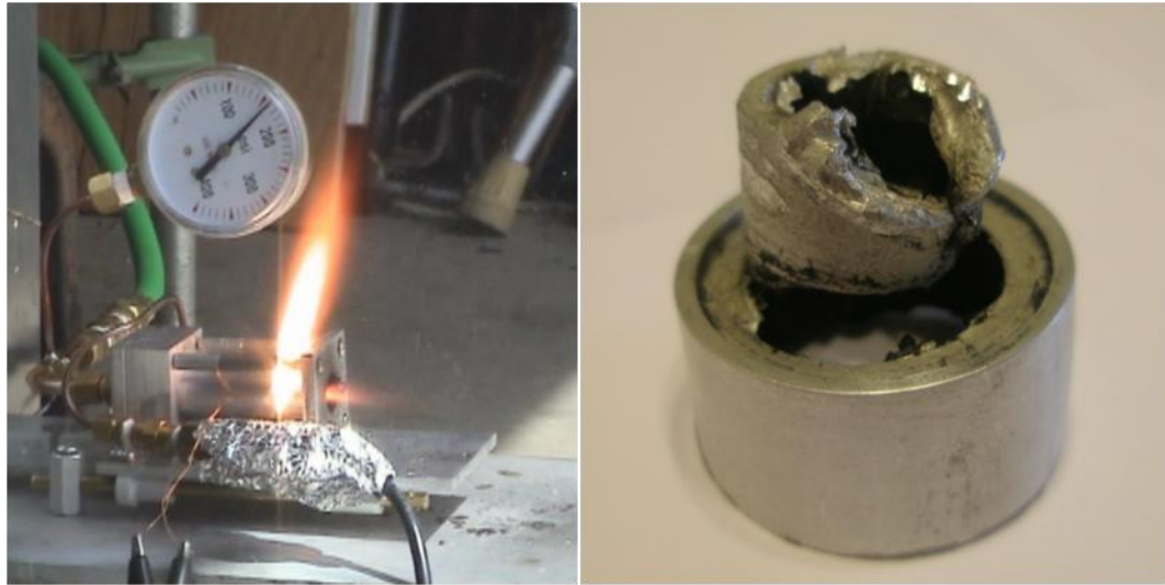
Fig. III-6 Motor failure with aluminum / graphite nozzle and resulting damage
