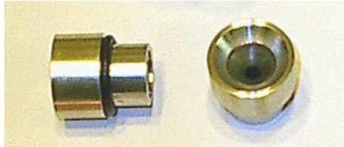
Fig. III-5 Machined aluminum nozzle with graphite insert throat
