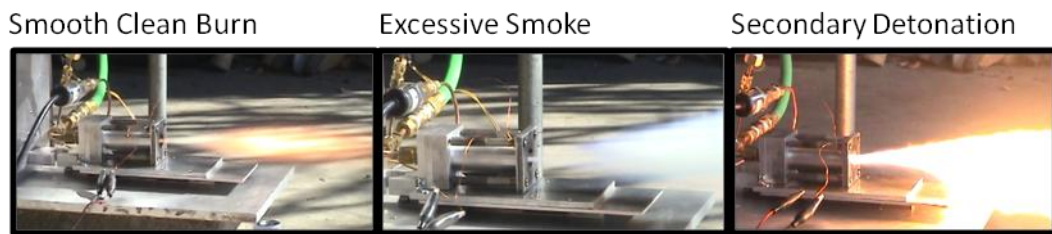
Fig. VI-7 Paraffin burns contrasting clean vs poor burns
