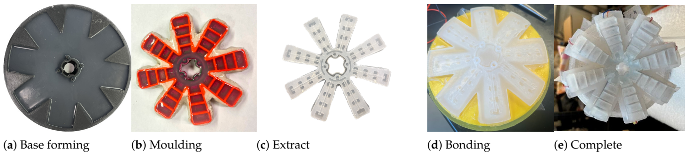
Figure 4. Fabrication process of the soft robotic pad with pneumatic fingers: (a) Pre-formed base seal for the pad; (b) mould for the pneumatic air chambers; (c) extracted model from the master mould; (d) bonded base to the pneumatic fingers; and (e) completed air chambers and pneumatic channels.
