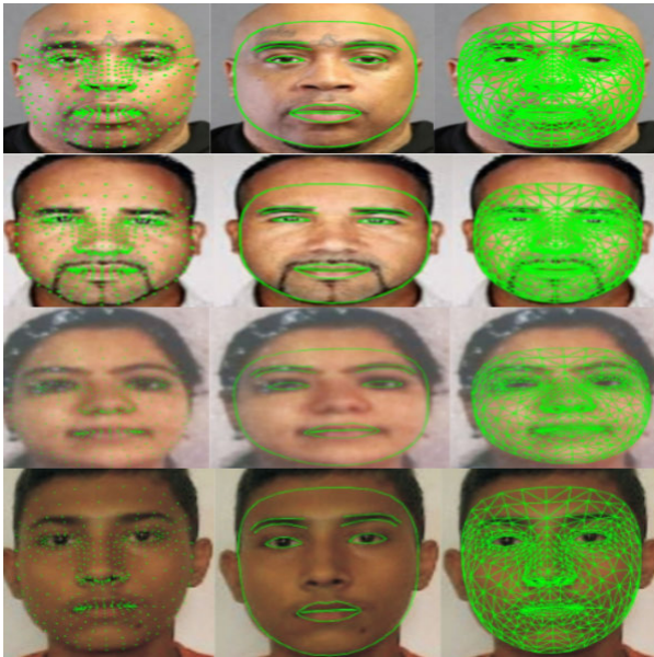
FIGURE 4. Overlaying of 468 landmarks on facial images [60], [61], [62], [63] of the self-created dataset and face mesh generation from the extracted landmarks.
